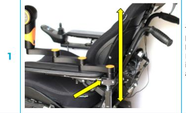
The attachment point has to be aligned with the shoulder, behind the armrest. If fitted on a mobile surface, it must be positioned as near as possible to the wheelchair.
