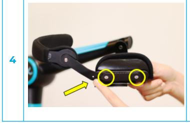
With the 2.5mm Allen key, lightly unscrew the 2 sliding bar's adjustment screws, in order to set the principal and the elbow support as far from one another as possible.
