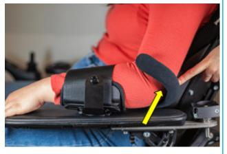
Put the elbow support closer to the arm until they are in contact.
