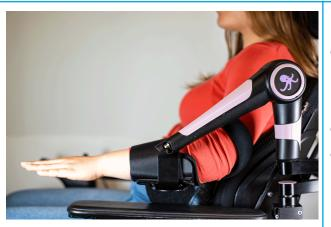
Choose the STATIONARY mode and with the buttons, position the arm brace a few centimeters above the armrest. The arm should be horizontal.
