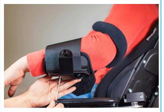
Tighten the 2 outer screws.
