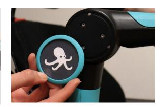
After removing the old image, place the new one inside, print side in front of plexiglas. Use the notch landmark to orientate it:
